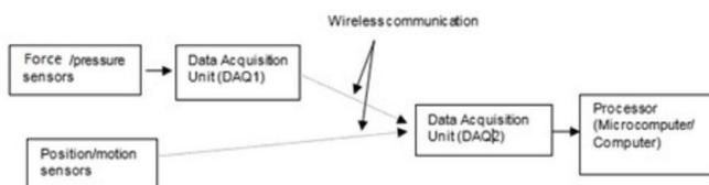
**Figure 1.** Block diagram of the mobile dynamic system
